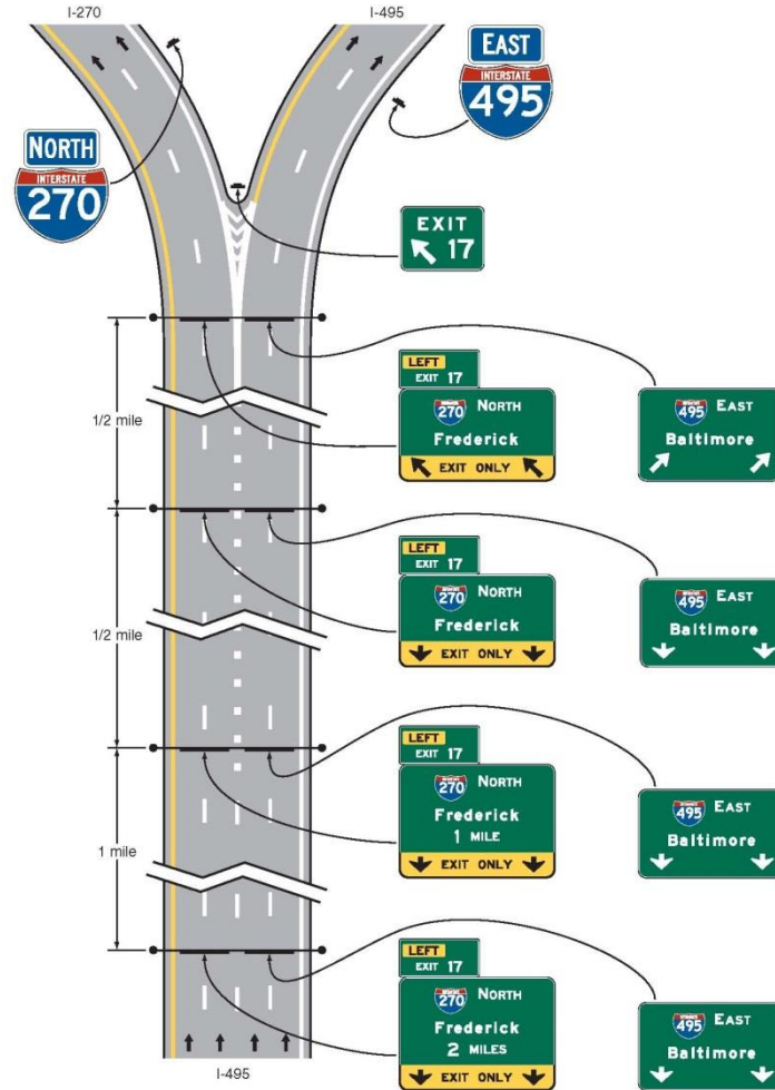
Figure 2E-14. Guide Signs for a Split with Dedicated Lanes
